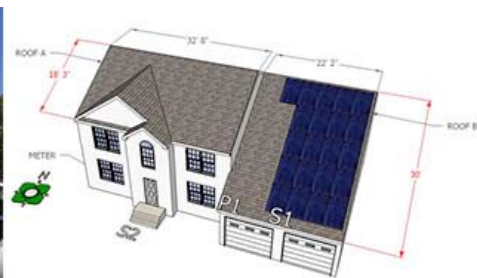
The actual system design showing 21 panels
